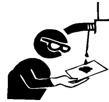
Using cardboard to check for oil leaks
